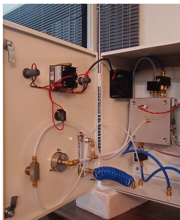
"A ceramic - based dielectric barrier discharge ozone generator, used for waste water treatment."
